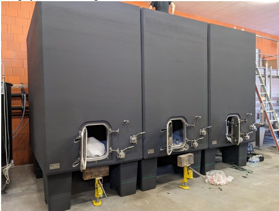
Using a jack for Shimming
