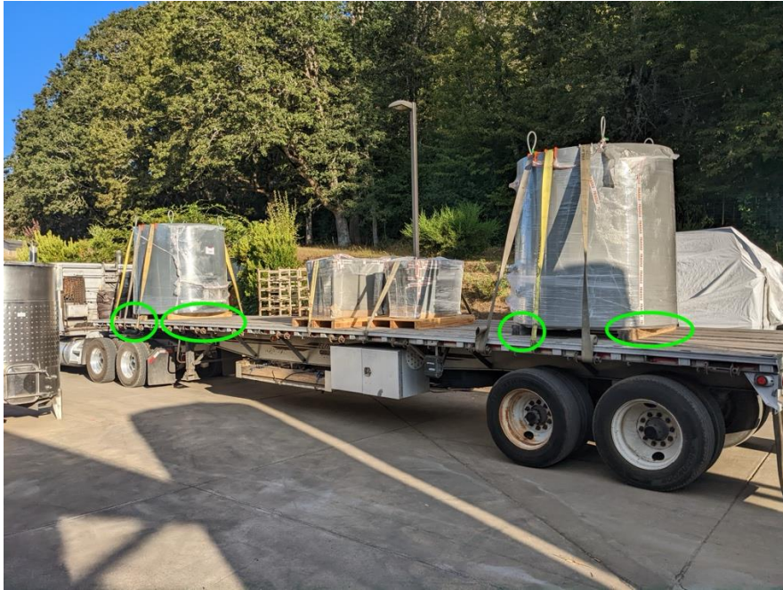
Anchoring for top of Feet – Included on pallet
