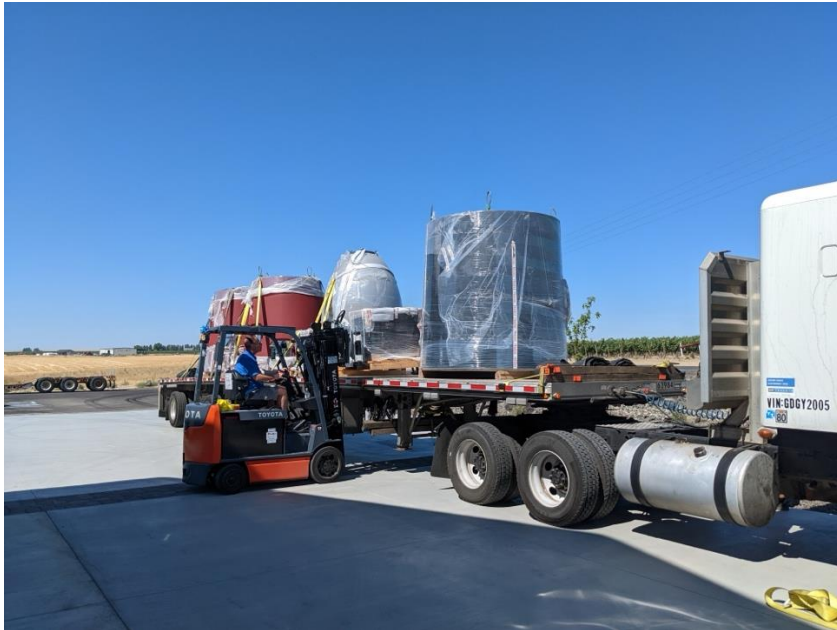
Offloading Pallet of Tank Feet (feasible with Standard forklift)
